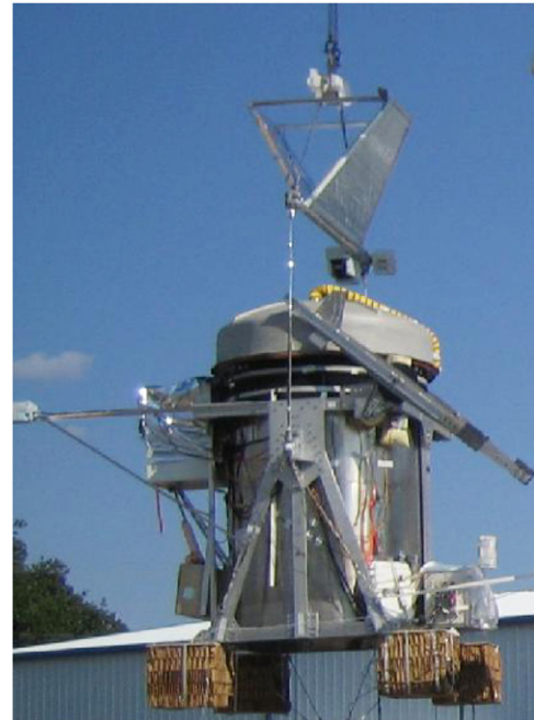
Figure 5. Photograph of the ARCADE 2 instrument just prior to 2006 flight. The instrument core is contained within the large (1.5 m diameter, 2.4 m tall) bucket dewar. The lid is shown closed for launch. The electronics box containing the warm stages of the radiometers and the payload electronics is mounted to the left of the dewar, and the three-axis magnetometers to determine orientation relative to the Earth’s magnetic field are seen to the left of the electronics box at the edge of the frame. The reflector plate is visible at the top of the photo above the lid. Cardboard pads at the four bottom corners absorb some of the impact when the payload hits the ground upon termination of the flight.
